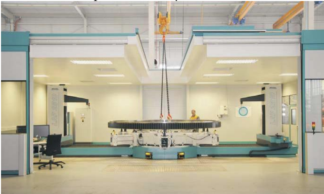
fig.1: double-sided coordinate measuring machine LAFD from Wenzel Präzision GmbH [1]
