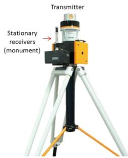
**Figure 2: Transmitter with stationary receivers**
