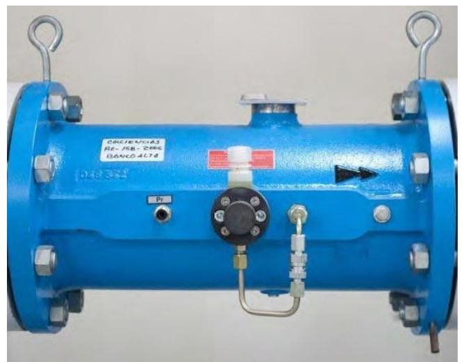
Fig. 4. The G-1000 turbine meter used as transfer standard
