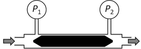
**Fig. 9. Longitudinal cross section of the annular LFM. The gas flowed through the small gap between concentric cylinders. The tapered end of the inner cylinder reduced turbulence in the gas exiting the gap. The inner cylinder used in the circular segment LFM cylinder had a similar taper.**
