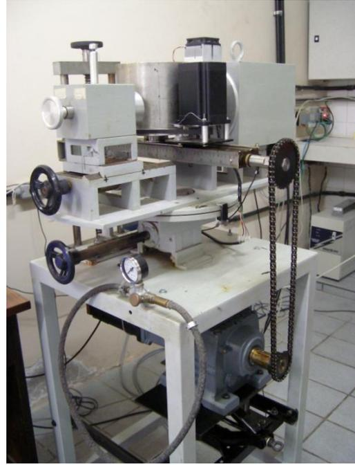
Fig. 1. Gamma ray scanner
