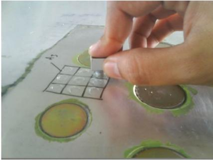
**Figure 2.5. Remaining thickness measurement by ultrasonic inspection. Several readings in a 10 x 10 mm grid.**
