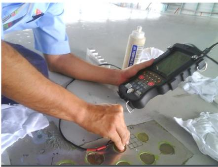
**Figure 2.6. Remaining thickness measurement by ultrasonic inspection.**
