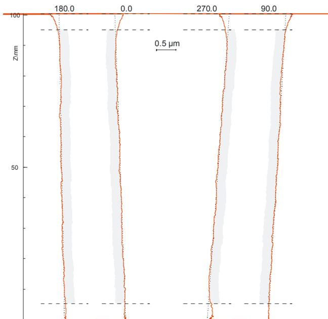
Fig. 5. Result of reversal procedure. The parallelism is corrected. The straightness is only influenced slightly.
