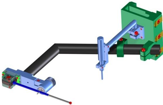
Fig. 3. Probe support with two arms and probes attached. The main support arm is made from CFRP.
