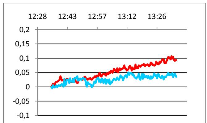
Fig. 7. Stability test with INVAR support: Red: laser read-out in  $\mu\text{m}$ , Blue: probe read-out. The stability of the INVAR support is much better than that of the current CFRP support. Horizontal axis is absolute time.
