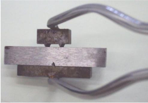
Fig. 4 – ASTM tongs for V-notched Charpy specimens.
