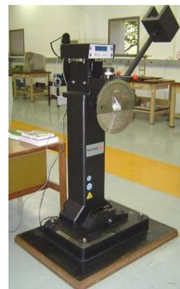
Fig. 3 – Instron-Satec Charpy impact testing machine. CETEC.
