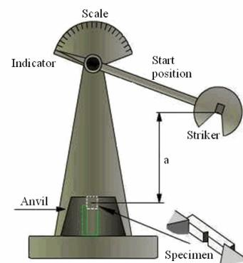
Fig. 2 – Energy measuring principles.
