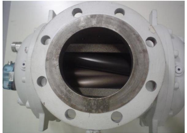
Figure 1 Delta S-Flow, G 250 rotary meter
