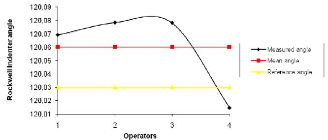
**Fig. 2. The behavior of the measurement of the angle of the indenter as a function of the operators**
