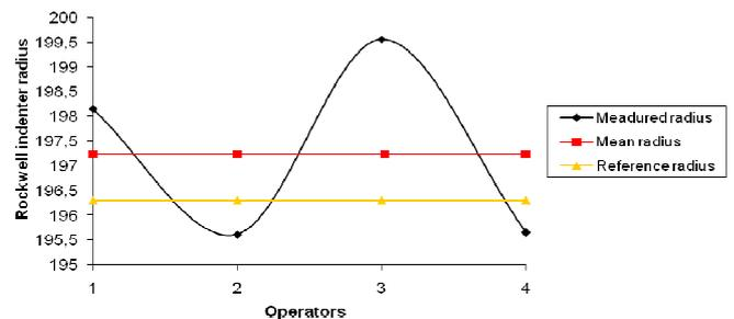
**Fig. 3. The measurement behavior of the radius of the indenter as a function of the four operators.**
