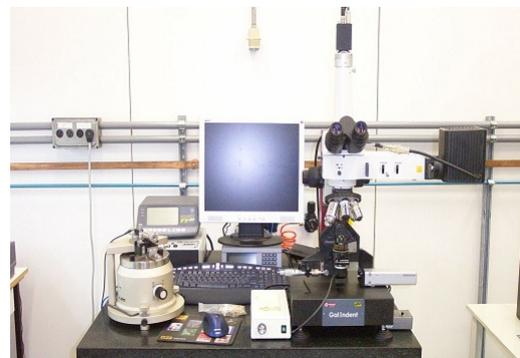
Fig. 1. Primary System of Rockwell and Vickers Diamond Indenters Calibration (Gal-Indent).
