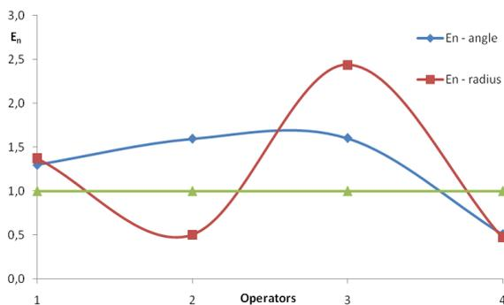
**Fig. 4. The normalized error for measurements of the angle (blue curve) and the radius (red curve) of the indenter as a function of each operator, as well as the compatibility limit for  $E_n$  (green curve).**
