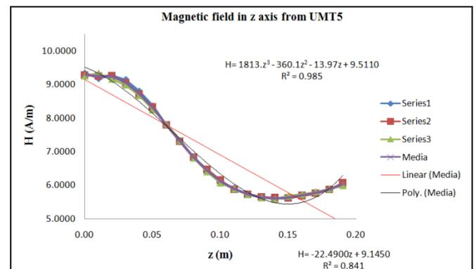
**Figure 6:** Magnetic field intensities along the vertical axis inside Mettler Toledo UMT5 mass comparator from Inmetro's Mass Laboratory.
