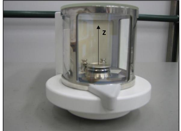
**Figure 2:** Vertical z axis centered on Mettler Toledo UMT5 mass comparator pan. Mass Laboratory – Inmetro.
