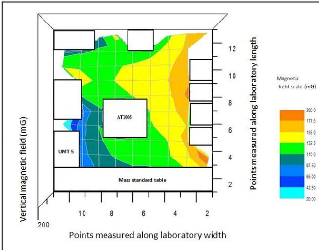
**Figure 3:** Magnetic field intensities measured in the circulation areas of the Mass Laboratory of Inmetro. Measurements were carried out at points in regular intervals of 0.5 m over the xy plane. Only the mass comparators under study are identified.
