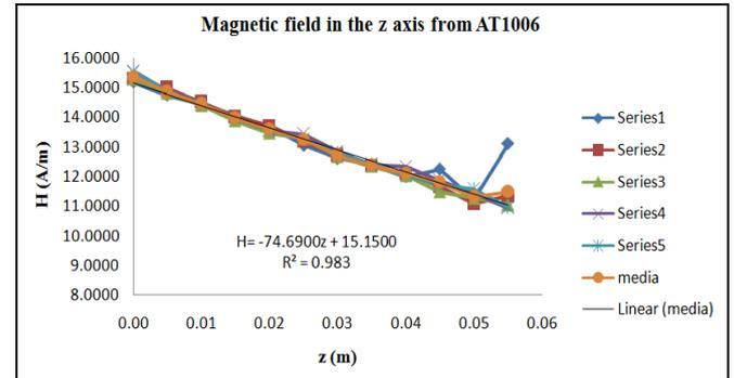
**Figure 5:** Magnetic field intensities along the vertical axis inside Mettler Toledo AT1006 mass comparator from Inmetro's Mass Laboratory.
