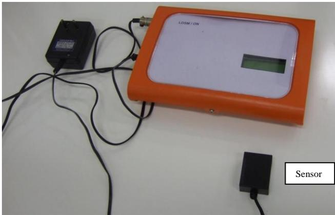
**Figure 1:** Magnetometer developed at LDSM/ON.
