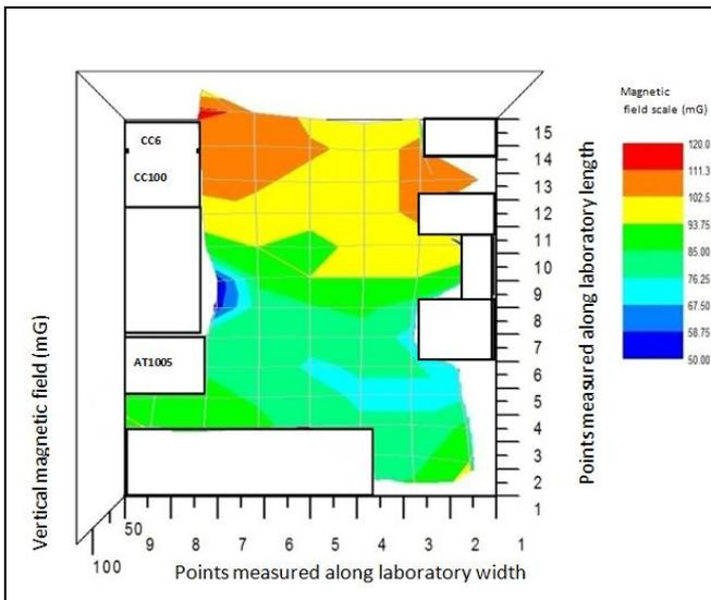
**Figure 4:** Magnetic field intensities measured in the circulation areas of the Mass Laboratory of LATU. Measurements were carried out at points in regular intervals of 0.5 m over the xy plane. Only the mass comparators under study are identified.
