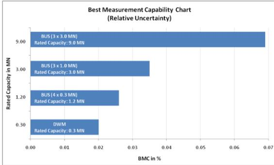
Fig. 2. Relative uncertainty for the corresponding measuring ranges (DWM: deadweight machine; BUS: build-up system)
