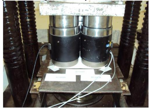
**Fig. 4. Complete three-load-cell-based build-up system during force machine calibration**
