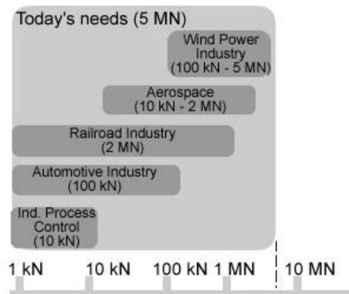
Fig. 1. Typical force measurement magnitudes for different business sectors - adapted from [3]
