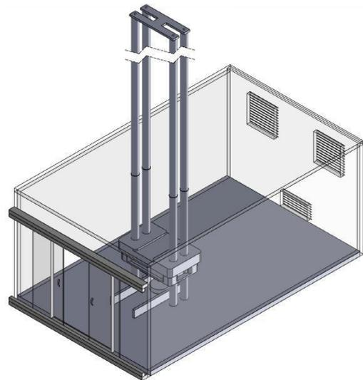
**Fig. 6. Sketch of the temperature-controlled room for the hydraulic force standard machine in order to improve calibration confidence**
