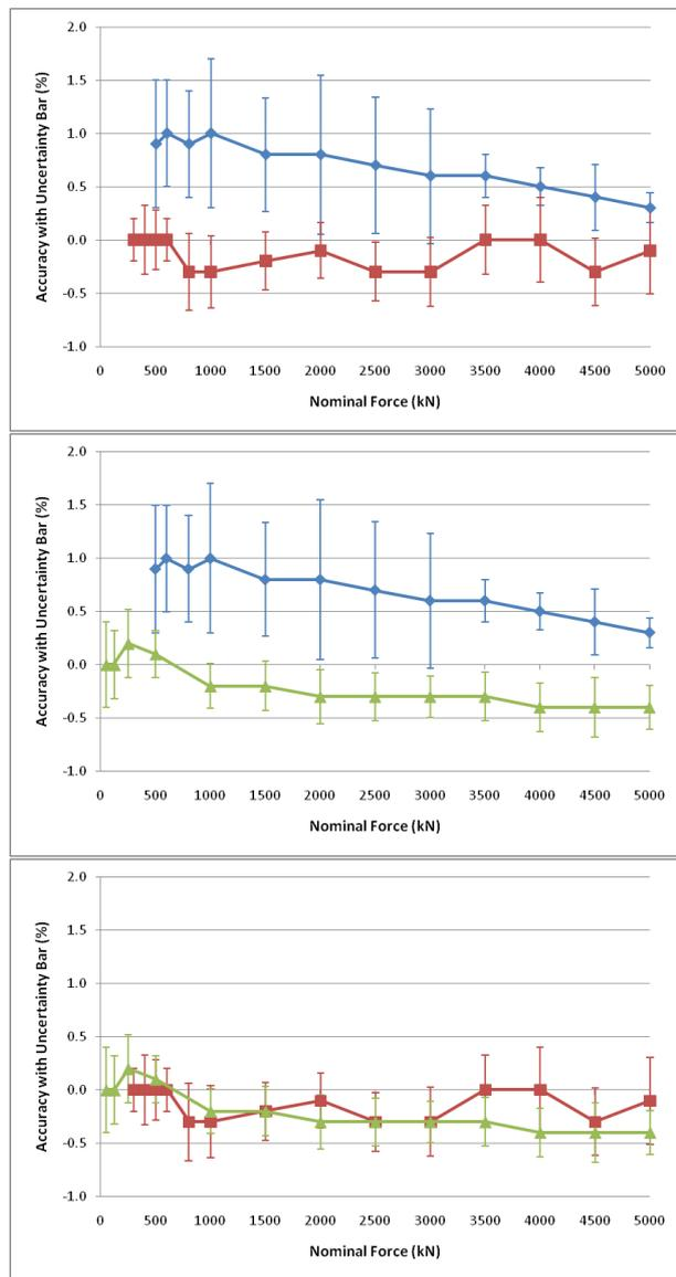
**Fig. 5. Machine calibration results for three different scenarios: (a) original machine (blue lines, diamond-type marker); (b) improved machine (red lines, square-type marker); (c) new build-up system setup (green lines, triangle-type marker)**
