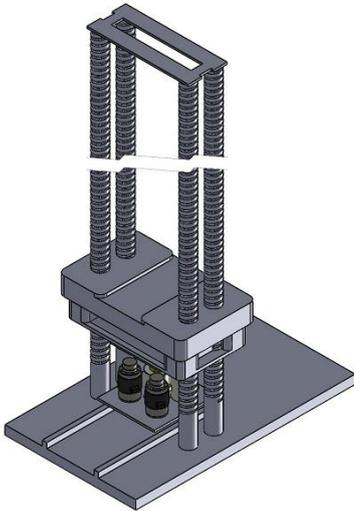
Fig. 3. Illustrative drawing of the hydraulic force standard machine with 5 MN nominal loading capacity
