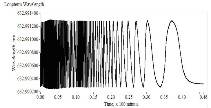
Fig. 2. Mode sweeping measured by wavelength meter.
