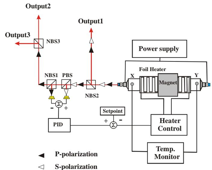
Fig. 1. Setup diagram for stabilized He-Ne laser system
