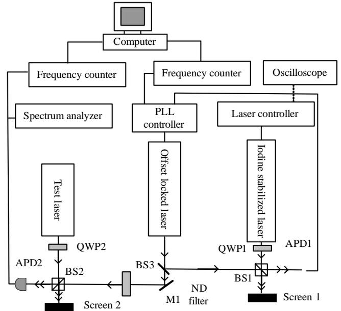
Fig. 6. The beat frequency measurement set up
