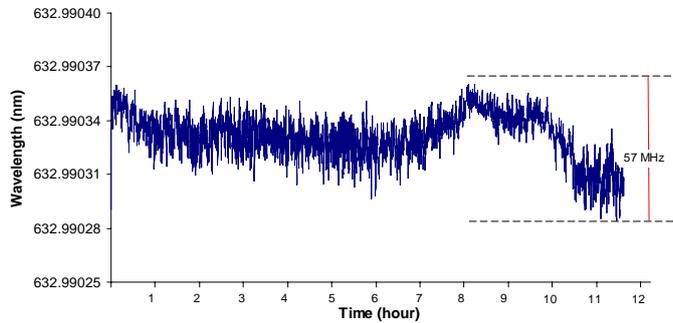
**Fig. 7. Long-term frequency stability of stabilized laser by using beat frequency technique.**
