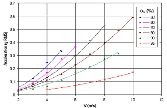
**Fig. 3. In-plane RMS acceleration in function of mixture velocity for different volume fractions of air.**
