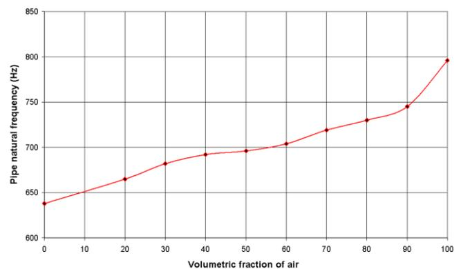
**Fig. 4. Variation of pipe natural frequency in function of air volumetric fraction.**
