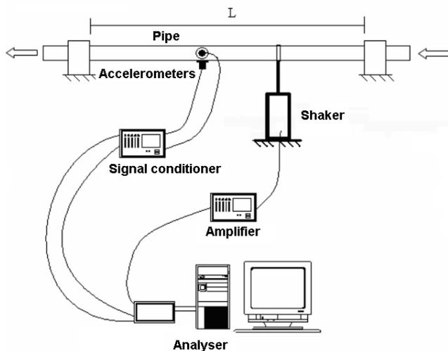
**Fig. 2. Experimental set up to obtain the pipe frequency response functions.**
