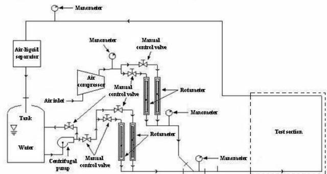
Fig.1. Schematic diagram of the air-water loop.
