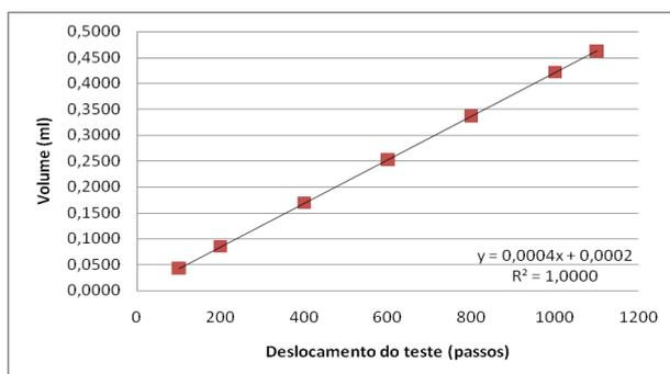
**Figure 06: Graph of the volume calculated by the weight of the volumetric flask.**
