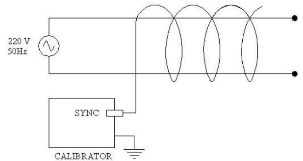
**Fig. 2 . Diagram for synchronization of impulses**
