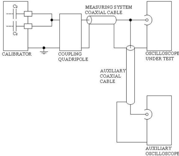
**Fig. 3 . Diagram for determination of impulse resolution time**
