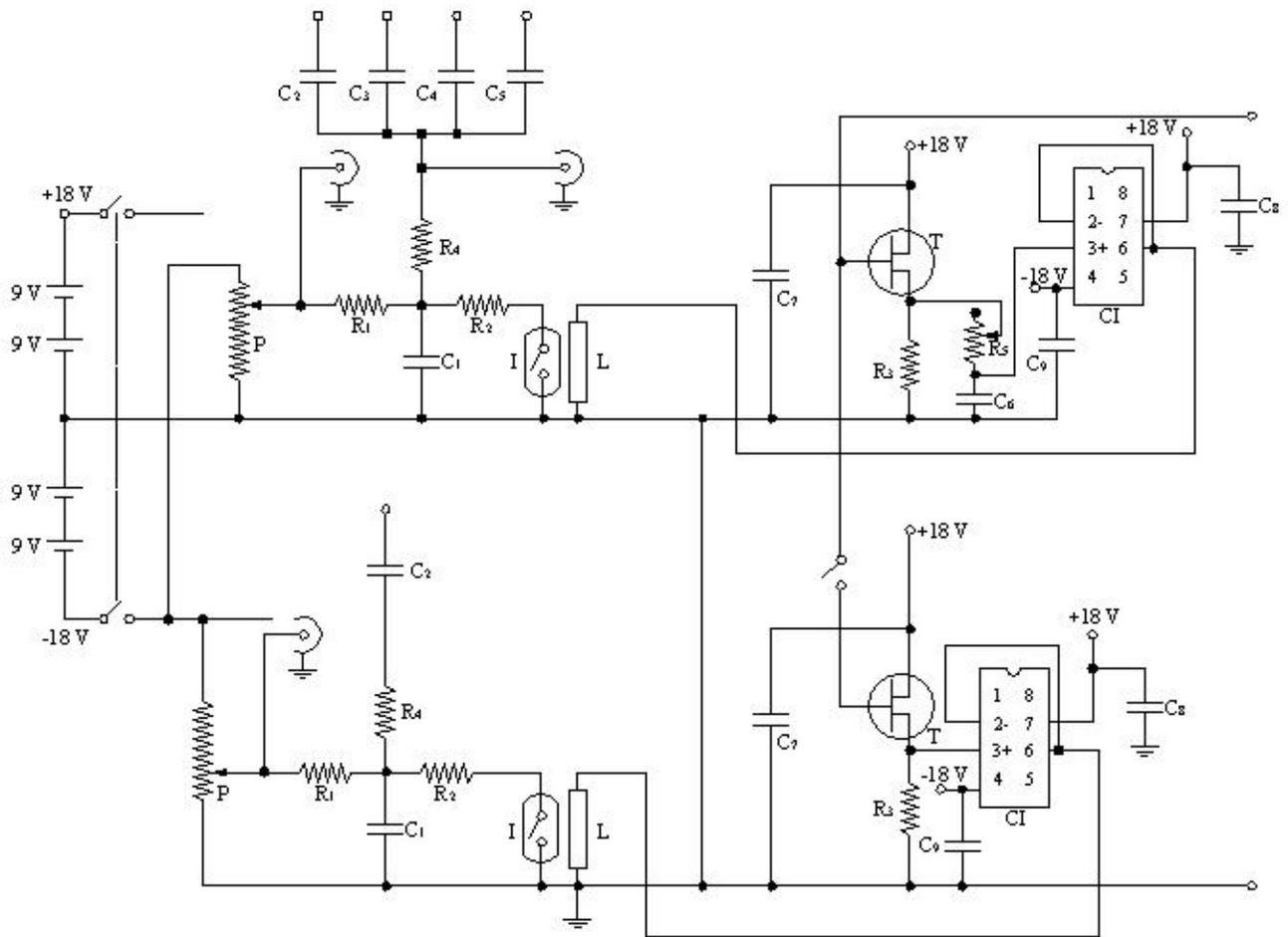
**Fig. 1 . Circuit of calibrator**
