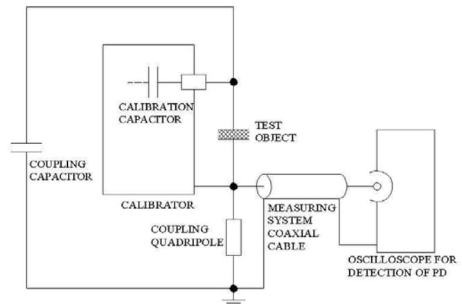
**Fig. 5 Diagram for determination of scale factor k (floating calibrator)**
