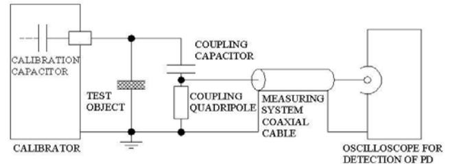
**Fig. 4 Diagram for determination of scale factor k (grounded calibrator)**
