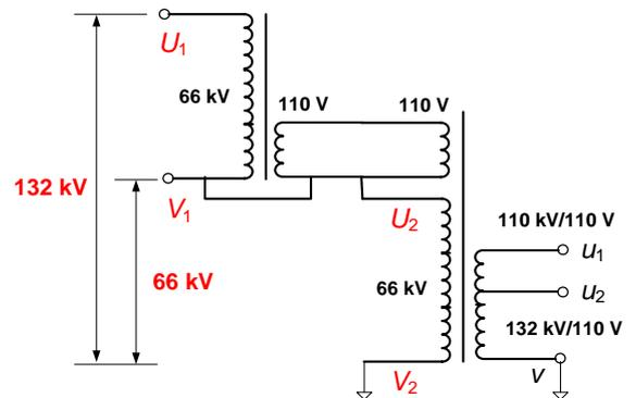
Fig.2. Basic circuit of the 132 kV PT
