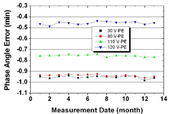
Fig.5. Phase Error of the 66 kV PT
