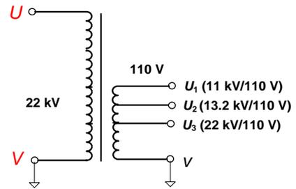
Fig.1. Basic circuit of the 22 kV PT
