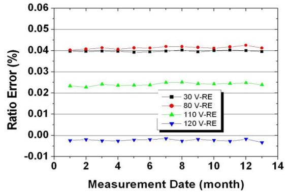
Fig.4. Ratio Error of the 66 kV PT
