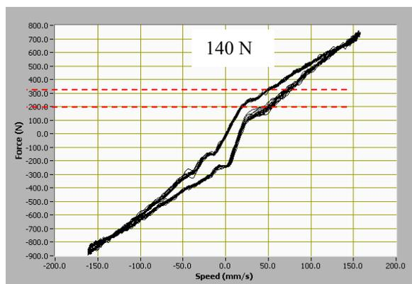
Figure 5 Force vs Speed characteristic of MR damper with hysteresis reduction.
