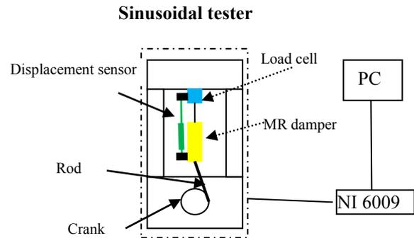
Figure 3 Block diagram of measuring stations and control
