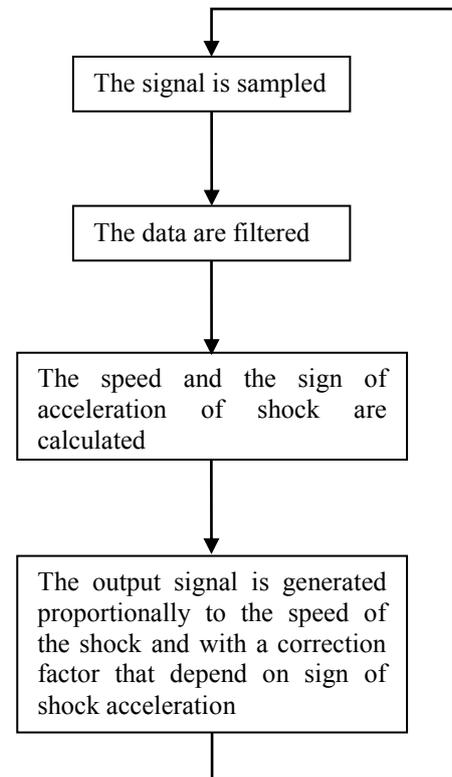
Figure 6 The block diagram of implemented algorithm.
