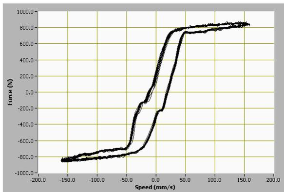
Figure 2 Force vs Speed characteristic of MR damper (with fluid MRF 132LD).
