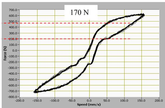
Figure 4 Force vs Speed characteristic of MR damper with hysteresis.
