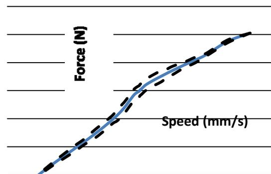
Figure 1 The damper curve characteristic [the real one (dashed), the mean one].
