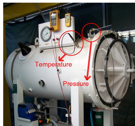
**Fig. 2. Calibration system for pressure**
