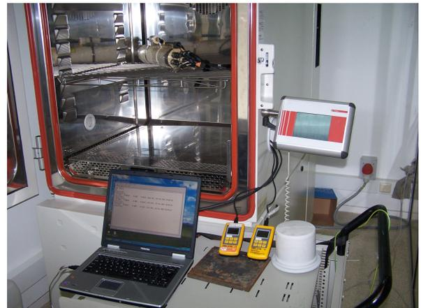
**Fig. 1. Calibration system for temperature**
