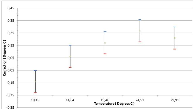
Fig. 4. Graph of the correction values with their expanded measurement uncertainty
