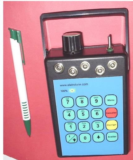
Fig. 5. Photograph of the ECG simulator prototype.
