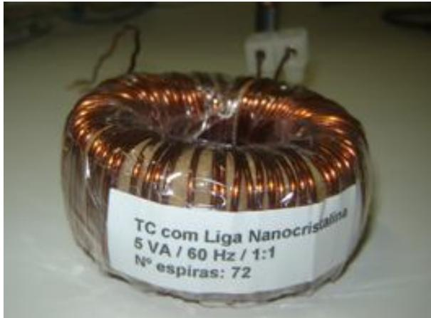
Fig. 3 – Prototype of current transformer
