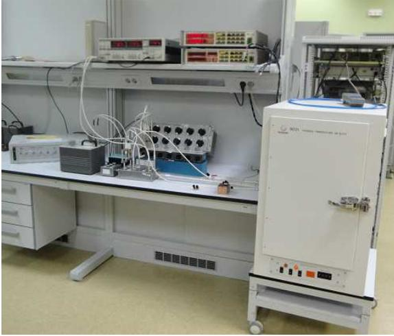
Fig. 3. General view of the Maxwell-Wien bridge.
