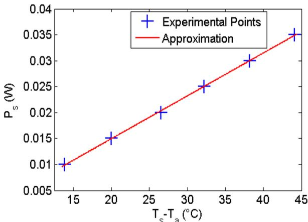
Fig 6.  $P_s \times T_s - T_a$  after transient, at each step of Figure 5
