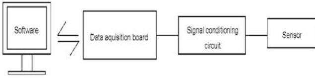
Fig 2. Experimental platform
