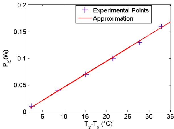
**Fig 9.  $P_s \times T_s - T_a$  after transient, at each step of Figure 8**
