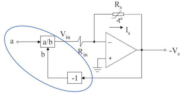
Fig 1. Basic electronic system with feedback linearization
