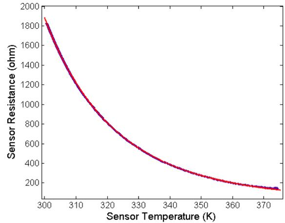
Fig. 7. Characteristic  $R_s \times T_s$ , sensor with encapsulation
