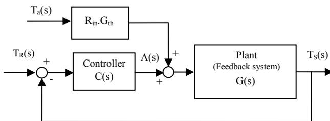
Fig 4. Block diagram of control structure
