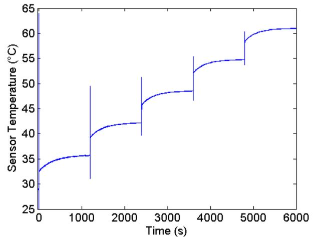
Fig 8. Staircase response to signal  $a(t)$  for a sensor with encapsulation
