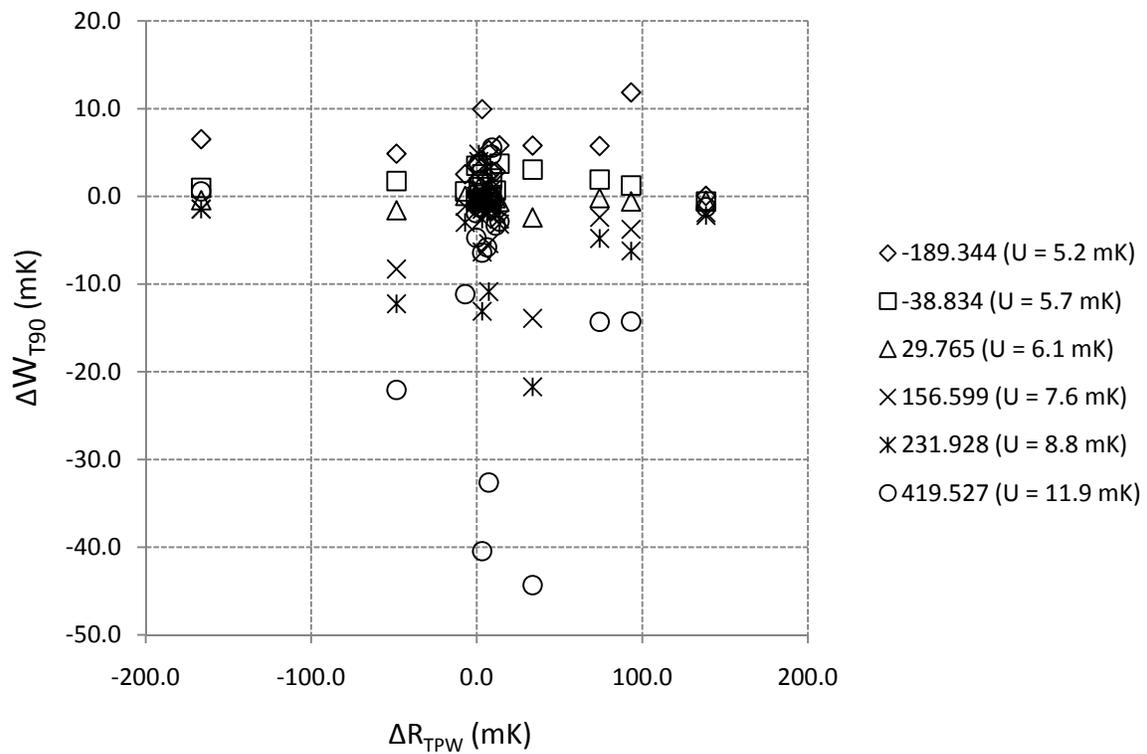
Fig.3.  $W_{T90}$  drift of 100  $\Omega$  secondary PRTs with different amounts of change in  $R_{TPW}$
