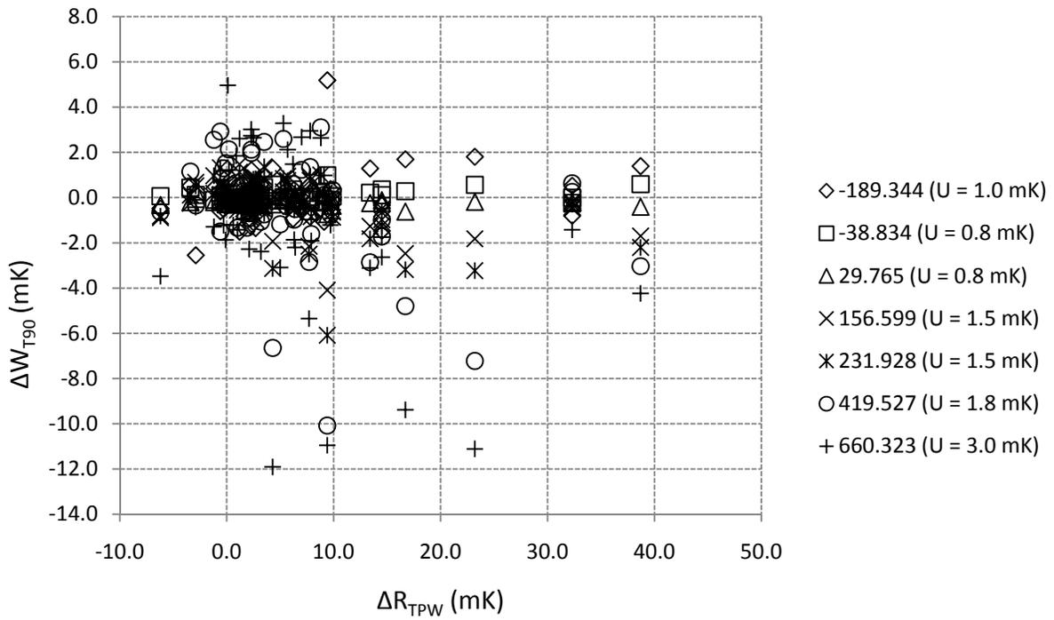
Fig. 1.  $W_{T90}$  drift of metal-sheath SPRTs with different amounts of change in  $R_{TPW}$
