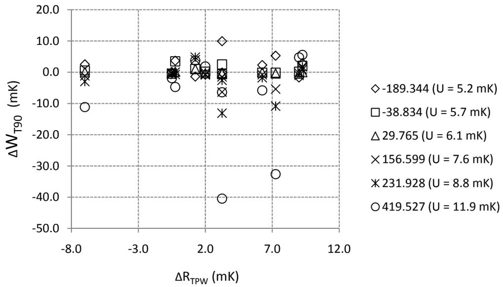
Fig. 4.  $W_{T90}$  drift of 100  $\Omega$  secondary PRTs with changes in  $R_{TPW}$  of less than 10 mK
