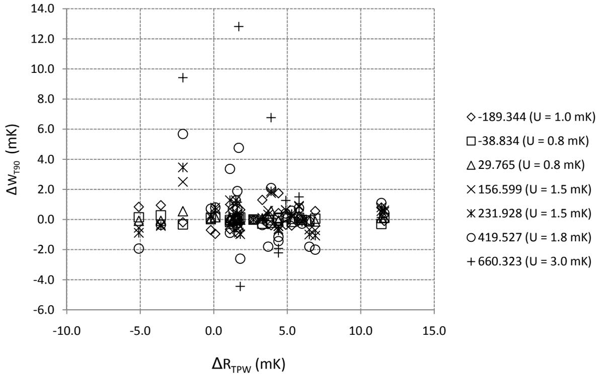
Fig. 2.  $W_{T90}$  drift of quartz-sheath SPTs with different amounts of change in  $R_{TPW}$
