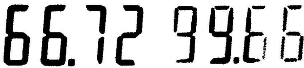
Fig. 2. Black and white output images over good lighting conditions (on the left) and over poor lighting conditions (on the right)
