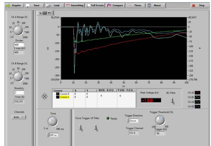
Figure 11. Main screen of the software.
