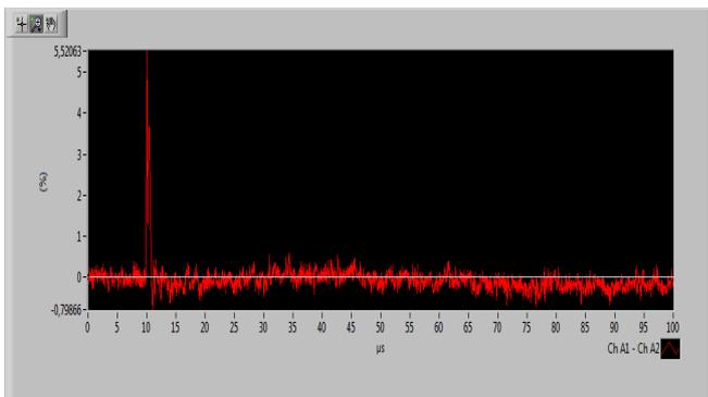
Figure 9 – Voltage comparison using the subtracting method.
