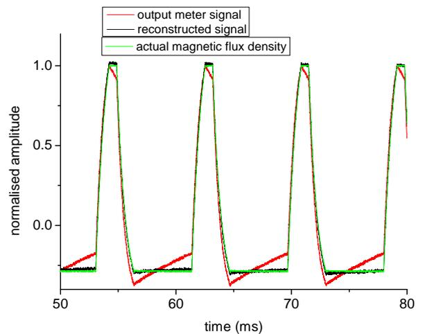
Fig. 15. Comparison between the actual magnetic flux density and the one reconstructed from the output meter signal.
