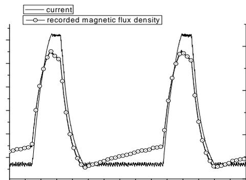
**Fig. 1. Comparison between current and magnetic flux density time behaviours simultaneously recorded during a welding operation.**
