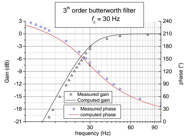
Fig. 8. Comparison between measured and computed gain and phase of the HPF with 30 Hz cut-off frequency.
