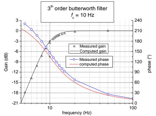
Fig. 7. Comparison between measured and computed gain and phase of the HPF with 10 Hz cut-off frequency.
