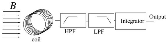
Fig. 2. Simplified scheme of a low frequency magnetic flux density meter, which includes the HPF and the low pass filter (LPF).
