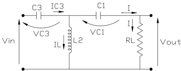
Fig. 12. Electrical circuit for the input voltage  $V_{in}$  reconstruction procedure.
