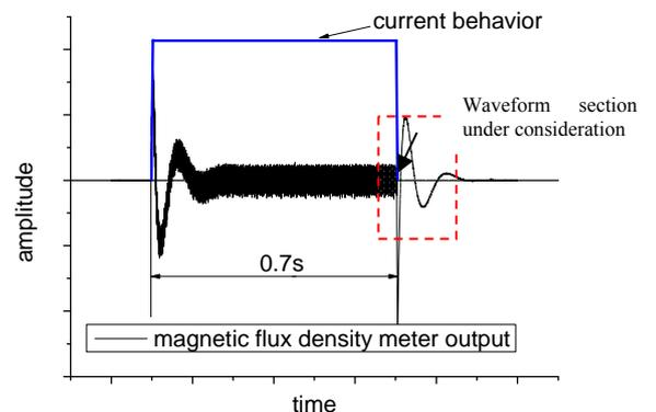
Fig. 10. Magnetic flux density detected near a cable supplied by a quasi-rectangular current.
