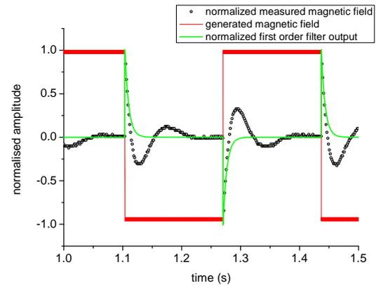
Fig. 4. Simulated and measured meter output signal under a rectangular magnetic field stimulus with a frequency of 3 Hz. All the quantities are normalized to their peak value.
