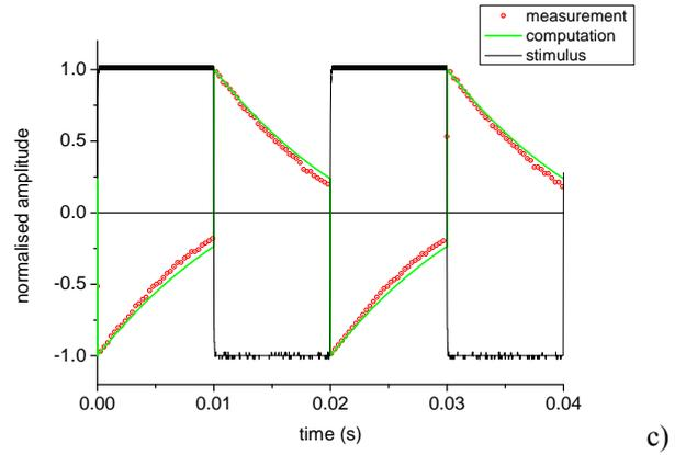
Fig. 9. Measured and computed meter outputs (values normalised to their peak), under a 3 Hz (a), 12 Hz (b) and 50 Hz (c) quasi-rectangular field.
