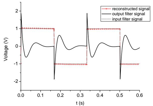
Fig. 14. Comparison between the enforced and reconstructed input filter signal.
