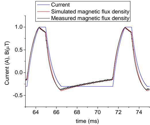
Fig. 3. Simulated meter output and measured magnetic flux density in the Helmholtz system supplied by the quasi-rectangular current.
