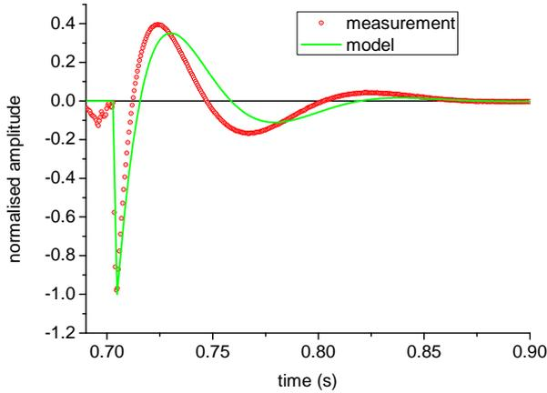
Fig. 11. Measurement and computation comparison for the free filter response.
