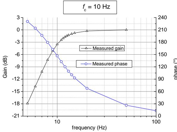
Fig. 5. Measured gain and phase of the meter transfer function versus frequency.
