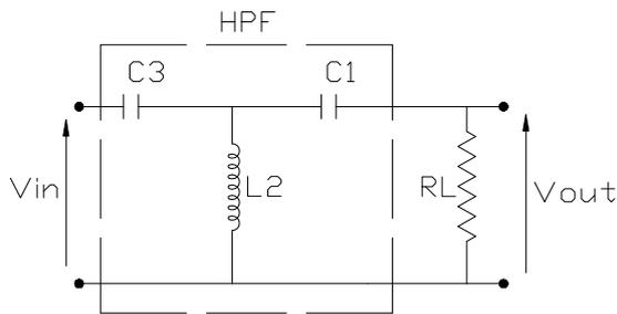
Fig. 6. Scheme of the HPF electrical model and the load (RL).
