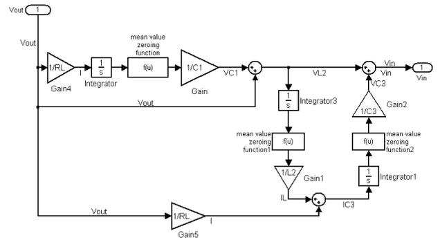
Fig. 13. Block scheme of equation solution
