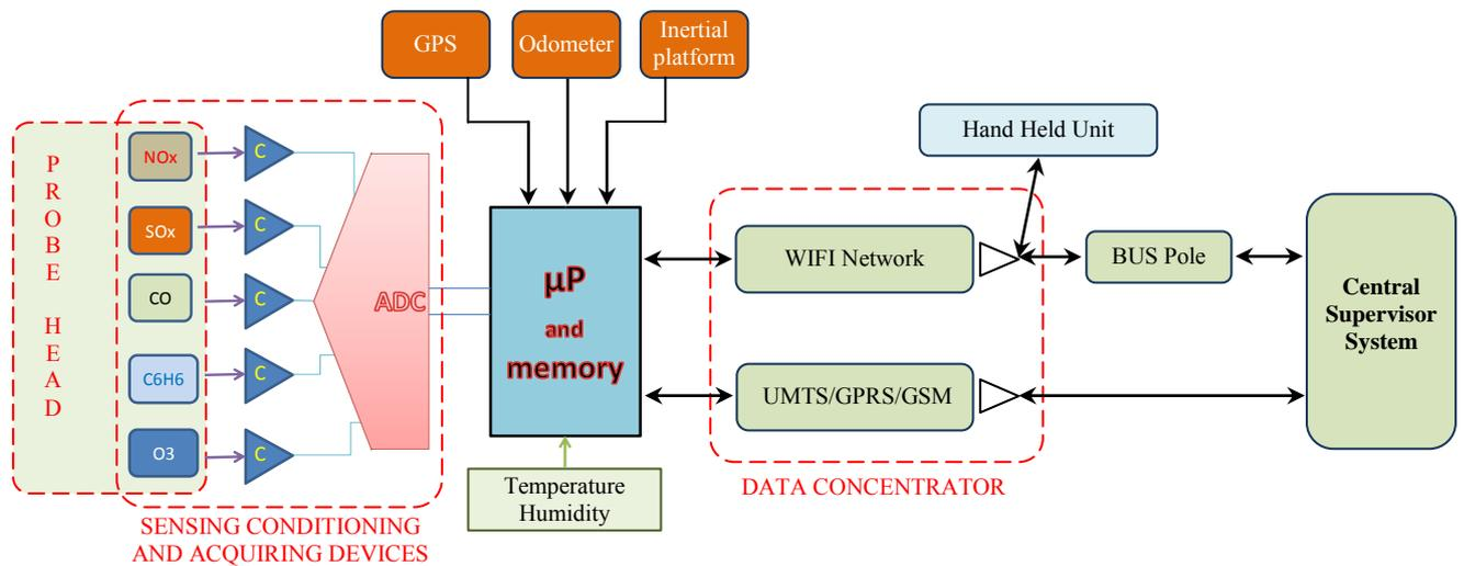
Fig. 2. Architecture of the proposed Mobile Measurement Unit
