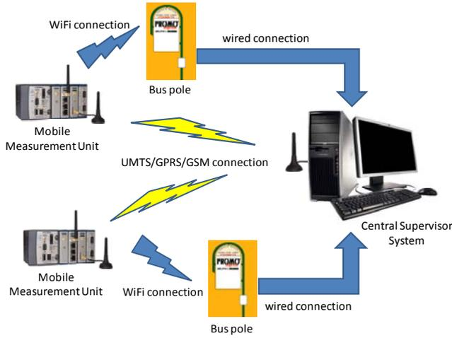
Fig. 1. General architecture of the measurement system
