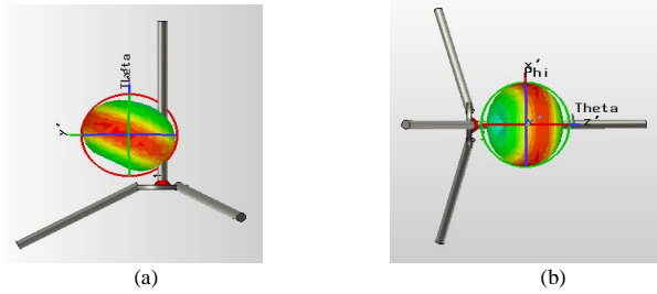
Fig. 3- Diagrams 3D of radiation monopole antenna simulated in the software CST: (a) Vertical, (b) Horizontal
