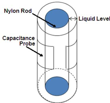
Fig. 9. Annular flow calibration scheme.
