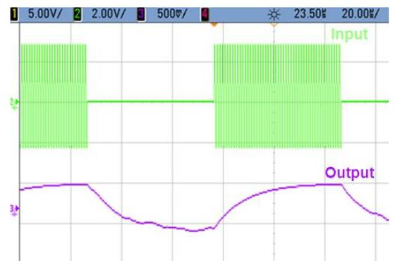
Fig. 4. Rise time of the system. Input signal on top and output at bottom.
