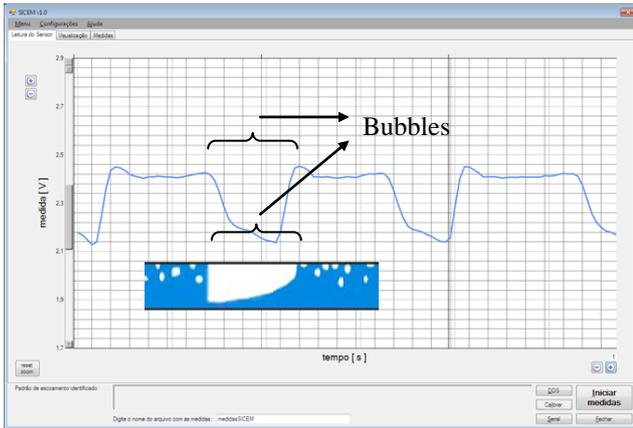
Fig. 6. A picture of the software during slug flow measurements.
