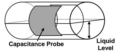
Fig. 7. Stratified flow calibration scheme
