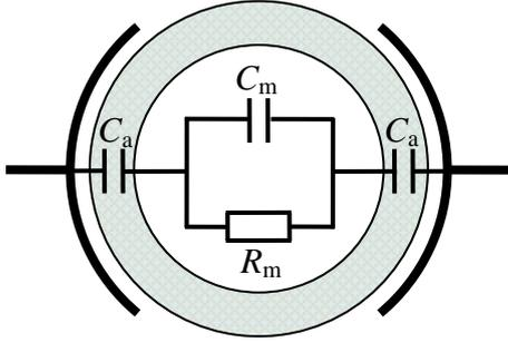
Fig. 2. Equivalent Electric Circuit of the capacitive sensor.
