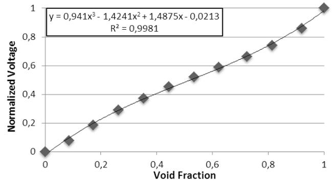
Fig. 8. Calibration line relating the normalized output voltage with the void fraction value.
