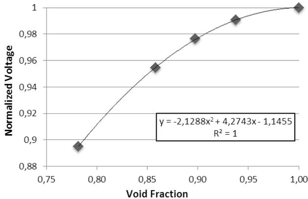
Fig. 10. Calibration line relating the normalized output voltage with the void fraction value.
