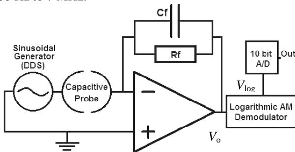
Fig. 3. Schematic diagram of measuring circuit
