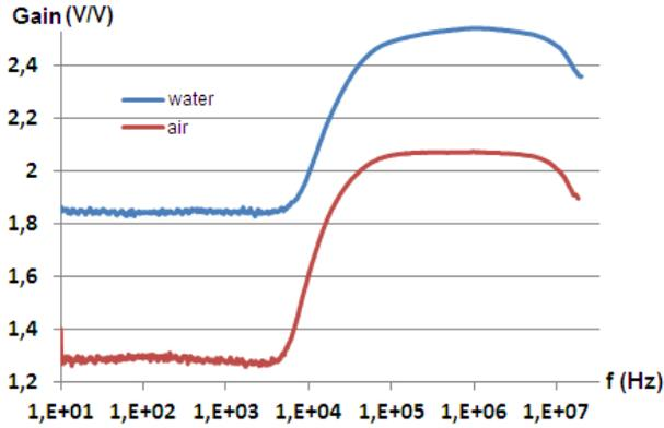
Fig. 5. Frequency response of the system. Curves for the sensor full of water on top and full of air at bottom.
