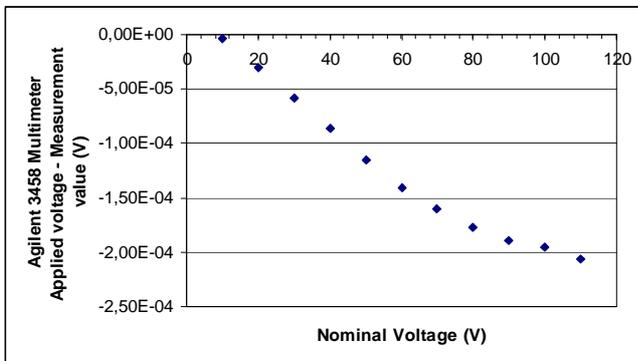
Fig.3: Calibration results for the DMM HP 3458A
