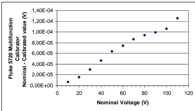
Fig.2: Calibration results for the multifunction calibrator Fluke 5720A
