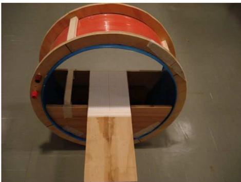
Fig. 4. Coil for field calibration Magmeter
