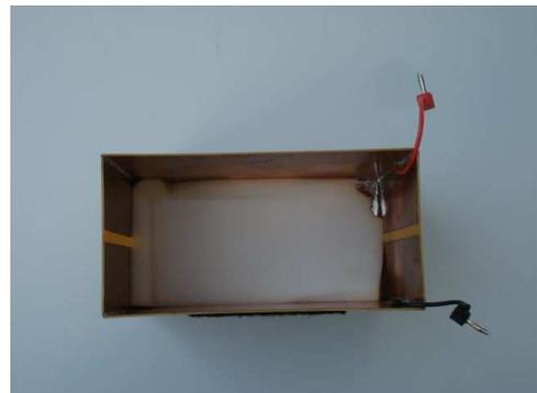
Fig. 1. The meter developed based on a capacitive sensor
