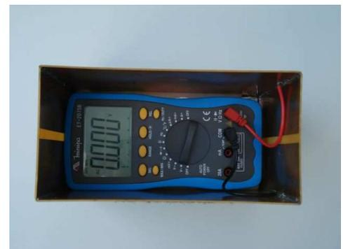
Fig. 2. The meter developed based on a capacitive sensor
