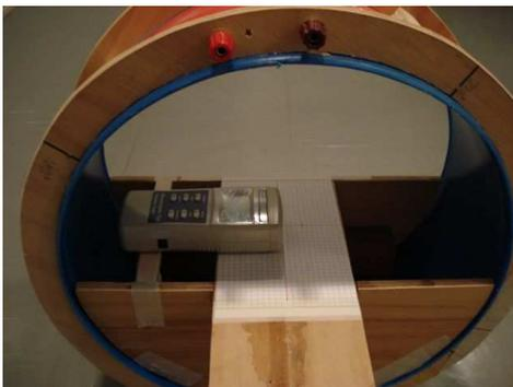
Fig. 5. Magmeter inside the coil for calibration
