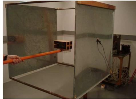
Fig. 6. Parallel plates for calibration of electric field.
