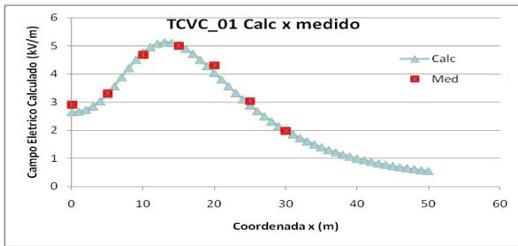
Fig. 3. Comparison of field simulation with the value measured on a 69kV line
