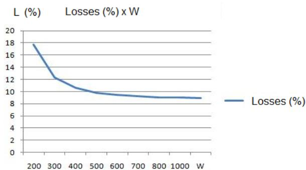
Figure 5: Switch loss in % for W, for  $L = 1,4$ ,  $V_{Store} = 20V$ ,  $V_{res}=10V$ .
