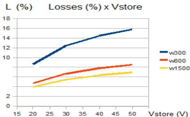
Figure 10: Circuit losses in relation to Vstore tension for different transistor size.
