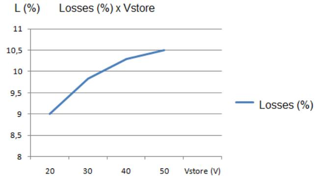
Figure 6: energy loss due to variation of  $C_{store}$  tension
