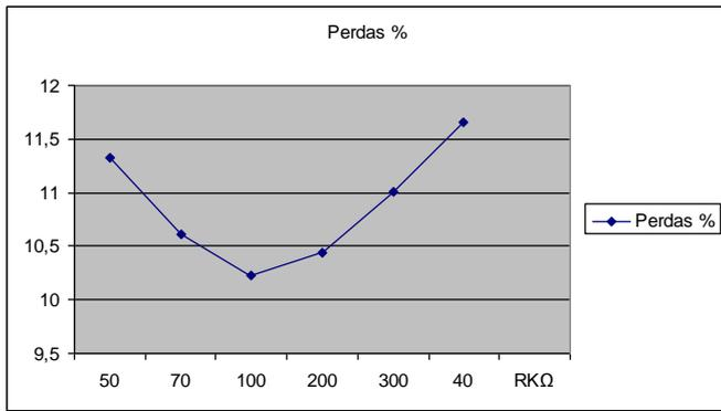
Figure 8: Switch losses in function of R1 resistance
