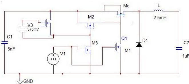
Figure 9: Circuit of the changed switch
