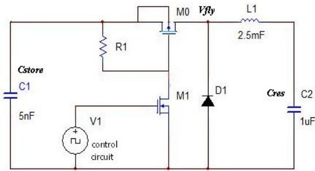
Figure 3: Control switch circuit
