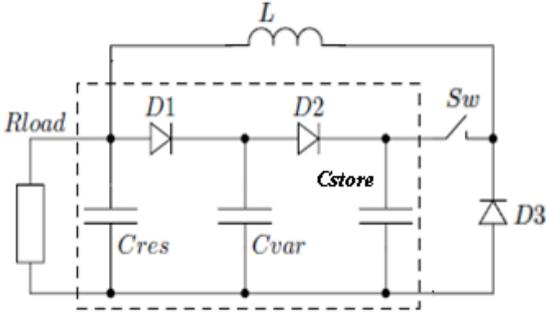
Figure 1: Circuit for Energy Harvesting
