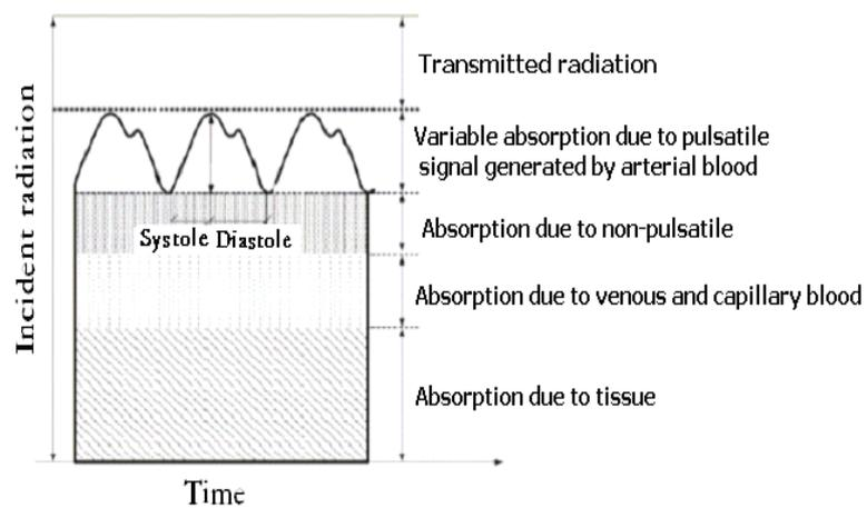
Fig. 1. Physical Principle of Pulse Oximeter – (a)
