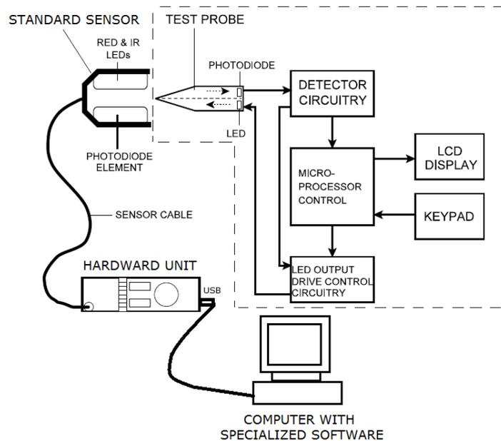
Fig. 6. Design of Pulse Oximeter Simulator Calibration Equipment
