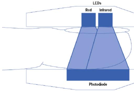
Fig. 3. LED Sensor of Pulse Oximeter
