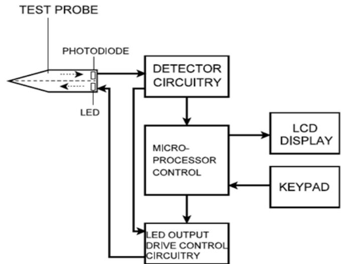
Fig. 5. Principle of Pulse Oximeter Simulator
