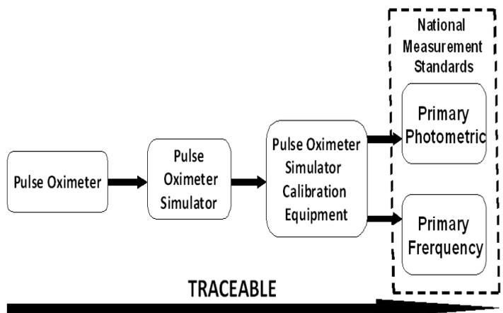
Fig. 7. Integrated Chain of Traceability
