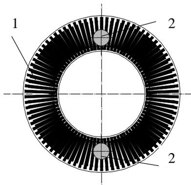
**Fig. 1.** Vernier fringe pattern formed by two circular raster scale. 1 – Vernier conjunction of two raster scales; 2 – photocells placed at opposite sides of the conjunction.
