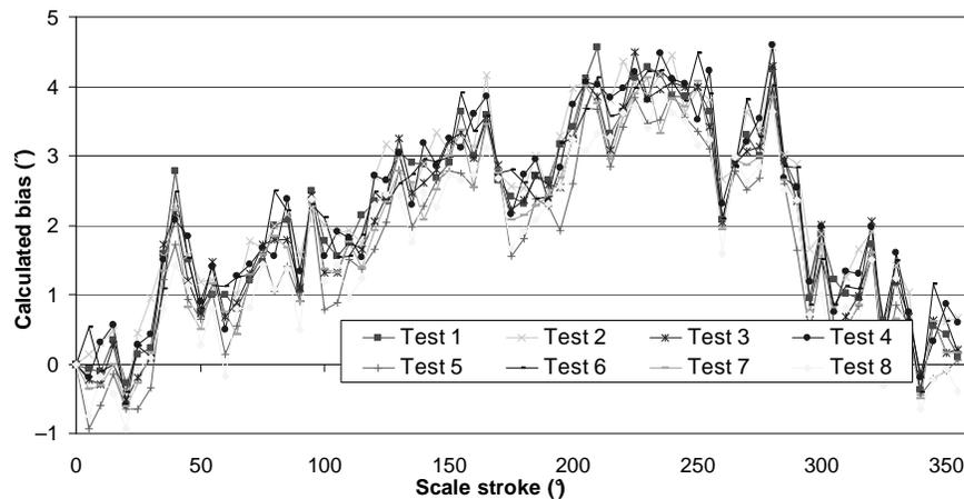
**Fig 2.** Systematic error of the circular scale recorded during the multiply measurement
