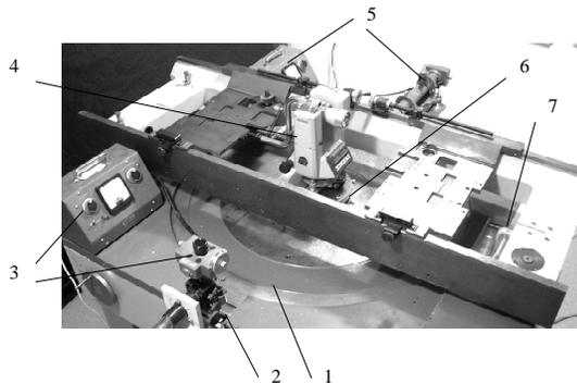
**Fig. 3.** View of the test rig for an angular measurements: 1 – worm wheel; 2 – circular scale on the wheel; 3 – photoelectric microscope with the display unit; 4 – geodetic instrument to be calibrated; 5 – autocollimator with the display unit; 6 – polygon; 7 – drive unit (step motor).
