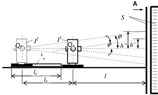
Fig. 5. Arrangement for vertical angle calibration of geodetic instruments
