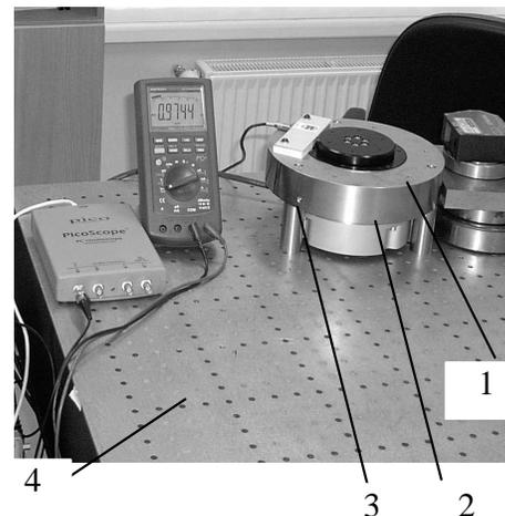
**Fig. 4.** Mechatronic rotary table for high precision angle measurements: 1 – the basis of the table, 2 – aerostatic bearing, 3 – piezoelectric drive.
