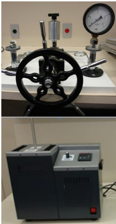
Figure 4. Dead Weight Tester and Dry Oven.
