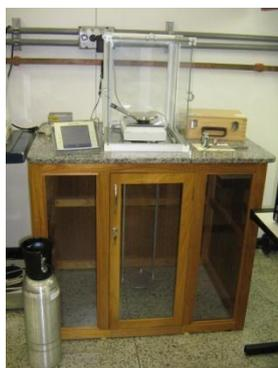
Fig. 2. – Mettler mass comparator balance
