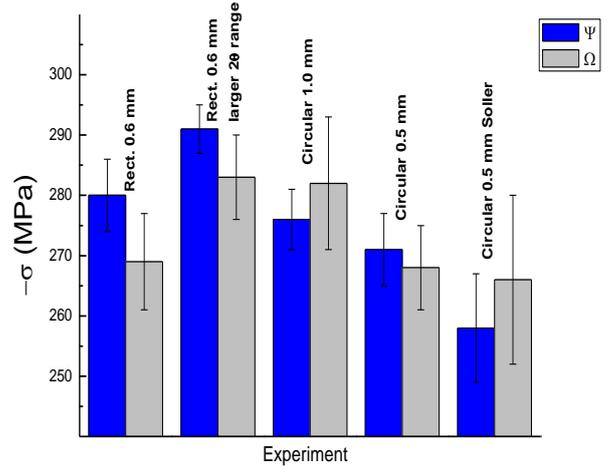
Fig. 3. Residual stress obtained in different experimental conditions
