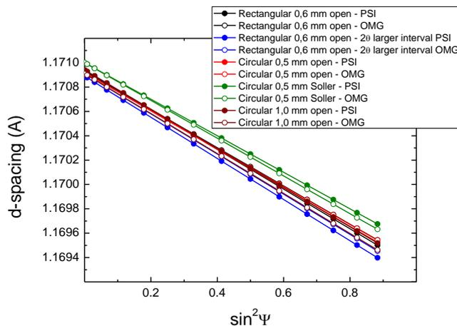
Fig. 2.  $d$ -spacing of (211) reflection planes as a function of  $\sin^2 \Psi$
