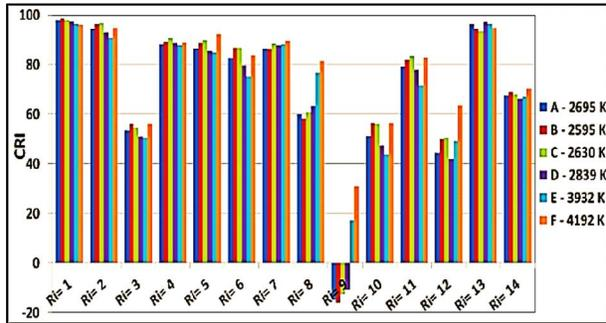
Fig.4. Set of fluorescent lamps of different color temperatures sampled in CRI, according the CIE standard in use [1].
