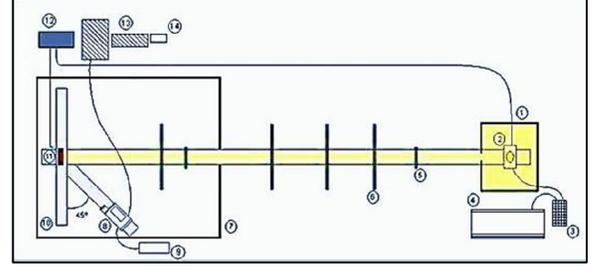
**Fig3. Experimental set-up;** (1),(2),(3),(4): “housing” and light source, standard resistance. (5), (6), (7): optical accessories and baffles. (8),(9),(10),(11): spectroradiometer, positioners, white tile. (12), (13),(14): computer, system measurements.
