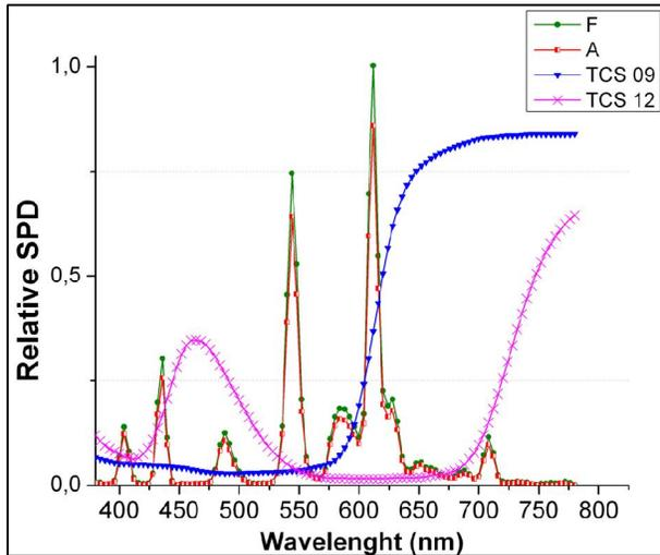
Fig.5. Spectral reflectance curve of CIE TCS 09 and relative SPD of test sources A and F.
