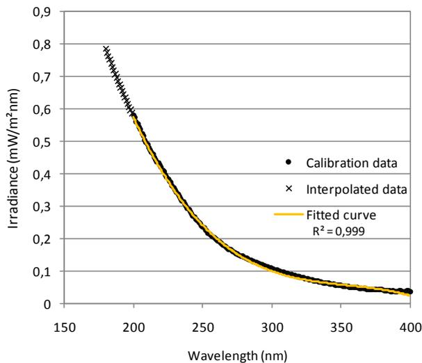
Fig. 2. Calibrated deuterium lamp irradiance data.
