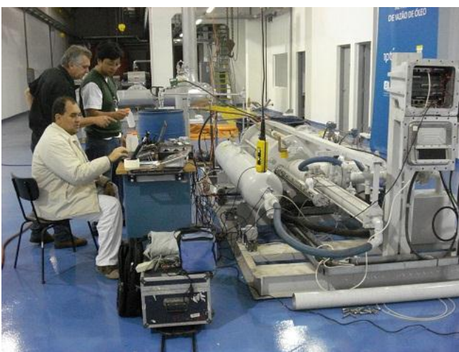
Fig. 12. Compact prover calibration by water draw method
