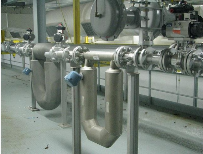
Fig. 6. Two Coriolis master meters used as working standards of the laboratory
