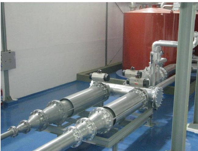
Fig. 8. Partial view of the test section including the telescopic connections to adapt the piping runs
