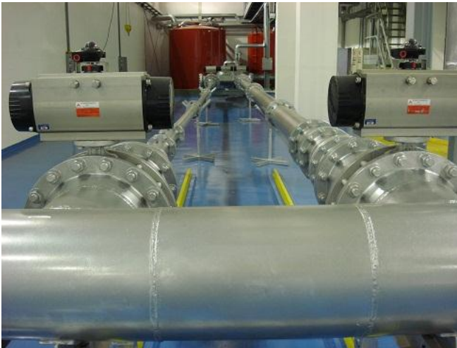
Fig. 7. General view of the test section including the two parallel test lines
