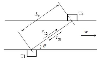
Figure 1: One path of a transit time ultrasonic meter.
