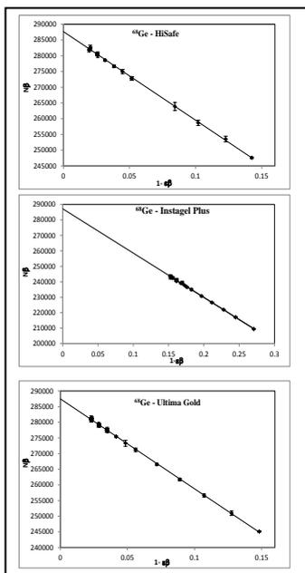
Figure 5. Extrapolation curve for each cocktail used in Anti-coincidence method.
