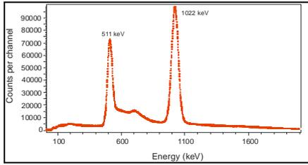
Figure 4. Spectrum obtained in the  $^{68}\text{Ge+Ga}$  sum-peak measurements.
