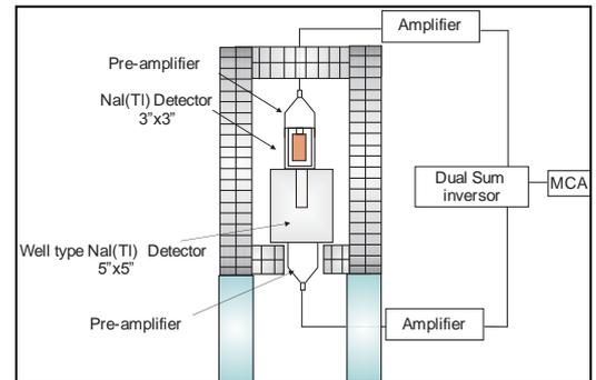
Figure 3. Experimental arrangement used in the sum-peak measurements.
