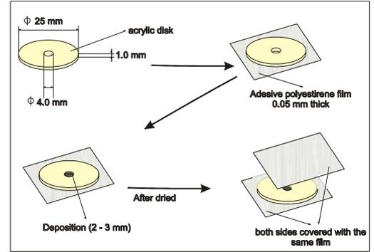
Figure 2. Preparation of the  $^{68}\text{Ge}/^{68}\text{Ga}$  sources.
