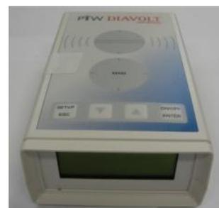
Figure 1: Non-invasive voltage meter PTW, Diavolt Universal All-in-one QC Meter model
