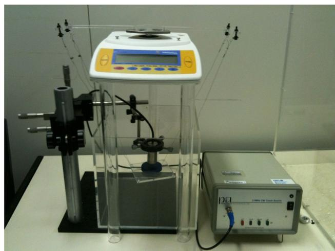
Fig. 1. Ultrasonic power measurement device: continuous wave check source, 3.5 MHz transducer, microbalance and assembly parts (no target is present).
