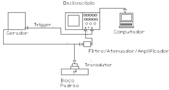
Figure 1. Experimental setup to determine the thickness measurement.
