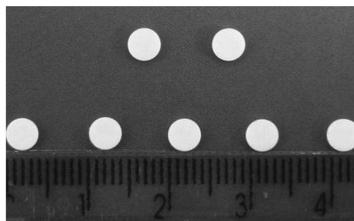
Fig. 1.  $\text{Li}_2\text{B}_4\text{O}_7:\text{Mn}$  dosimeters pellets in relation to a rule scale (cm).
