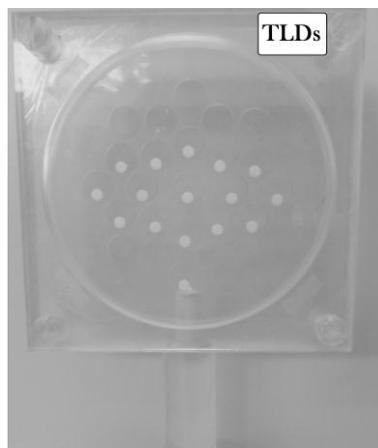
Fig. 2. Irradiation holder of the TL dosimeters.
