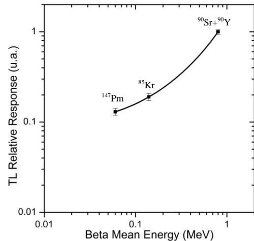
Fig 5. Energy dependence of the detectors exposed to beta radiation sources (BSS2 system).
