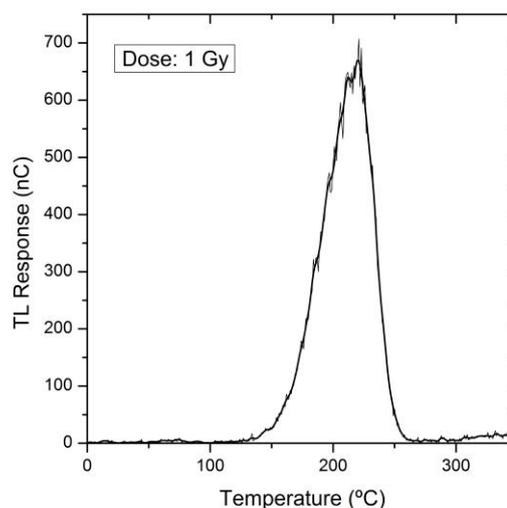
Fig. 3. TL glow curve of a  $\text{Li}_2\text{B}_4\text{O}_7:\text{Mn}$  pellet irradiated with 1 Gy of  $^{90}\text{Sr}+^{90}\text{Y}$  (BSS1).
