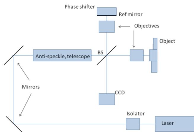
**Fig. 1.** Set up of Linnik type interferometer, where BS is the high quality 50/50 beam splitter, Object is the step height or master height standard, Objectives are the conformal pair of x10, x20 microscopic objectives. Ref mirror is the reference mirror optionally located on phase shifting PZT module.
