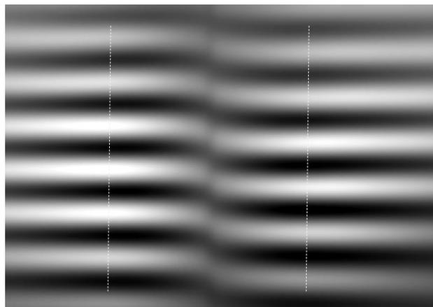
Fig. 3. Fringe pattern for 10 um GB step taken with Linnik interferometer. Vertical dashed lines are the eye guide used to select digitized area of the pattern.
