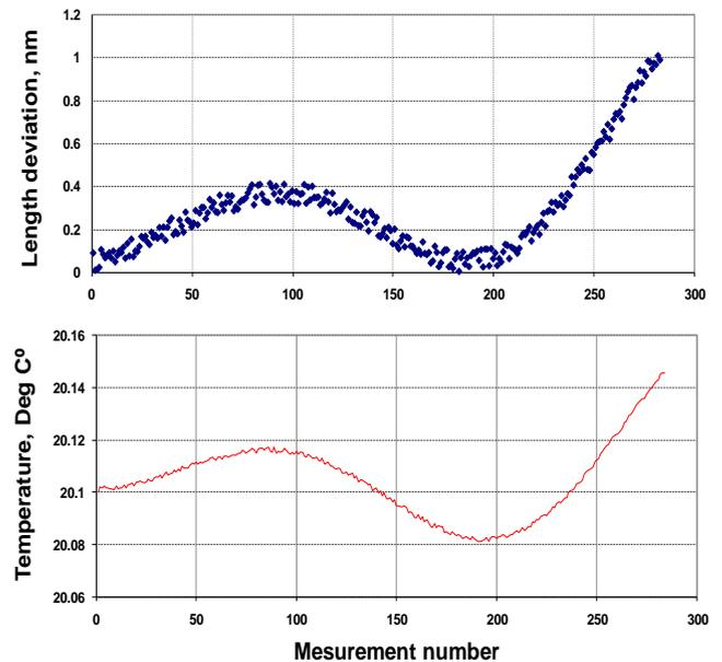
Fig. 6. Correlation of the temperature drift with measured length. About 300 measurements performed during several hours of continuous read out.
