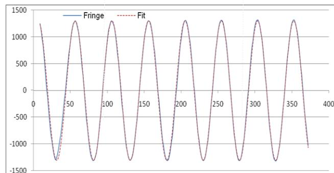
Fig. 4. Quality of the fringe (solid) and the fit (dash). Typical difference in most of the pattern is less than 1% almost invisible. Pixel number on X axis, the relative intensity of the CCD image on Y axis.
