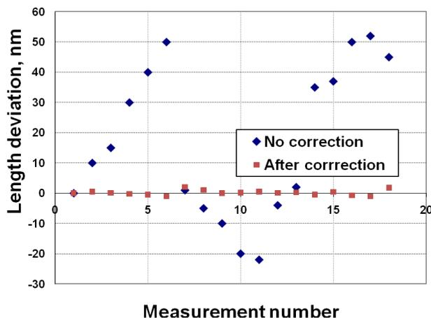
Fig. 7. Misalignment error of interferometer. Several measurements non-corrected and after correction. Standard deviation of the corrected values is about 0.8 nm.
