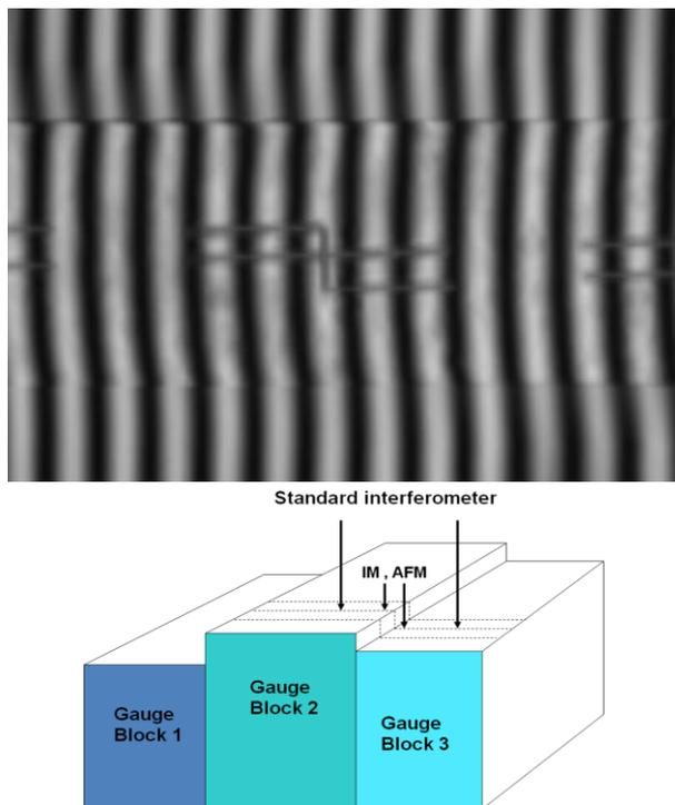
Fig. 2. Interferogram of triple GB standard. On the bottom is the layout of the triple GB step Master Standard.
