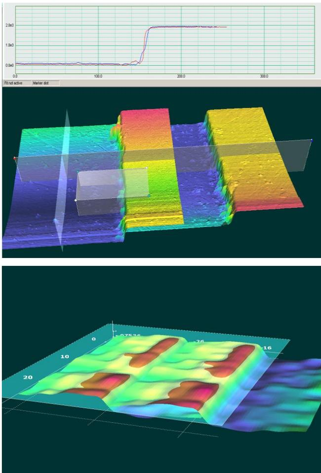
Fig. 5. Comparison of the data with AFM comparator 3D mode. Interactive Cube is used to mark the area of interest for parameter calculation. Planes are set to read intersection with corresponding 2D plots (upper part). At lower image Z intersection plane is used for detailed map comparison between 2 measurements.
