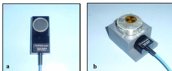
**Fig. 1. a) Superficial ionization chamber and b) chamber during the stability test, with the <sup>90</sup>Sr+<sup>90</sup>Y check source.**
