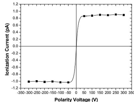
Fig. 4. Saturation curve of the ionization chamber.
