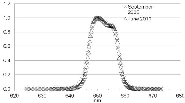
**Fig. 11. Relative spectral responsivity of the LP3 pyrometer at 650 nm measured in September 2005 and June 2010.**
