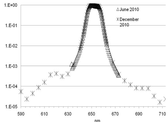
Fig. 3. Relative spectral responsivity of the LP3 pyrometer at 650 nm measured in June and December of 2010.
