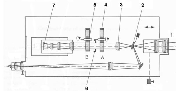
**Fig. 1. Optical arrangement of the LP3 pyrometer:** objective lens (1); measuring field stop (2); collimator lens (3); filter wheels A (4) and B (5); aperture stop (6) and detector (7).
