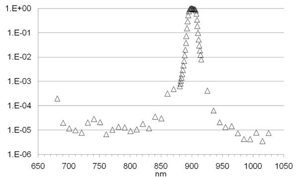
**Fig. 9.** Relative spectral responsivity of the LP3 pyrometer at 900 nm measured in December of 2010.
