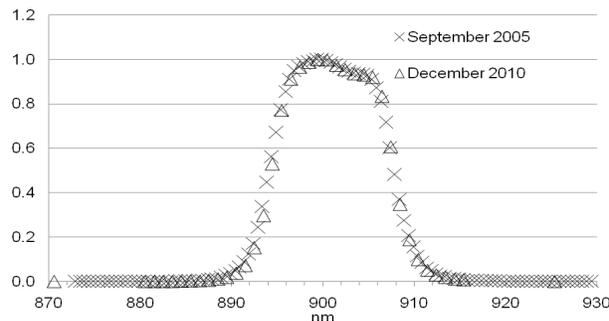
**Fig. 12. Relative spectral responsivity of the LP3 pyrometer at 900 nm measured in September 2005 and December 2010.**
