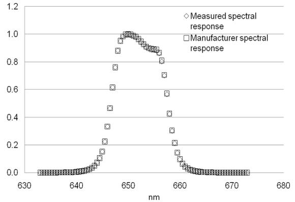
**Fig. 7.** Relative spectral responsivity of the LP3 pyrometer at 650 nm calculated as product of its components measured separately and using the manufacturer spectral response of photodiode.
