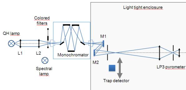
Fig. 2. Experimental setup for spectral responsivity.
