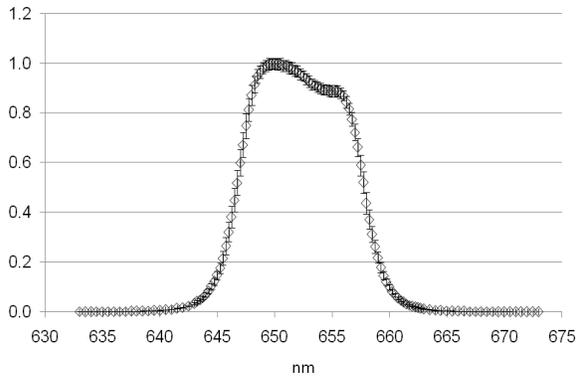
**Fig. 4.** Relative spectral responsivity of the LP3 pyrometer at 650 nm and associated expanded uncertainties measured in June 2010.
