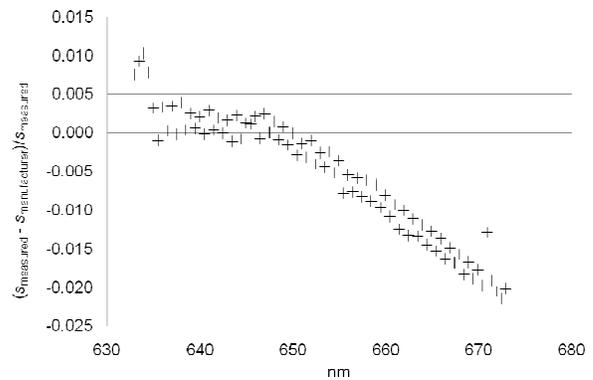
**Fig. 8.** Relative difference between relative spectral responsivity of the LP3 pyrometer at 650 nm calculated as product of its components measured separately and using the manufacturer spectral response of photodiode.
