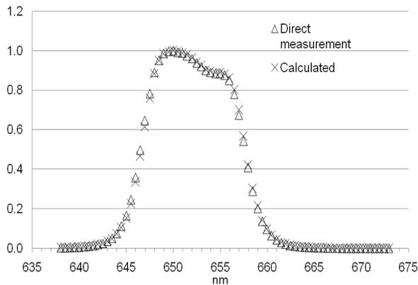
**Fig. 5.** Relative spectral responsivity of the LP3 pyrometer at 650 nm measured directly and calculated as product of its components.
