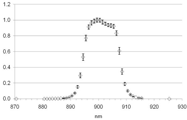
**Fig. 10. Relative spectral responsivity of the LP3 pyrometer at 900 nm and associated expanded uncertainties measured in December 2010.**
