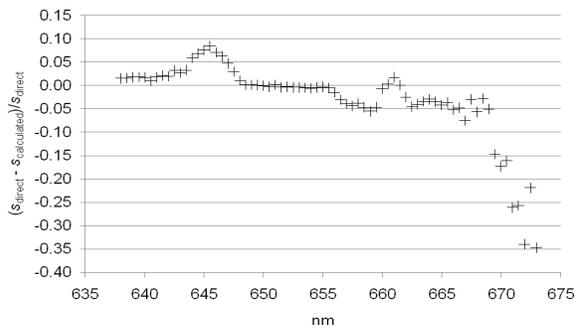
**Fig. 6.** Relative difference between relative spectral responsivity of the LP3 pyrometer at 650 nm measured directly and calculated as product of its components.
